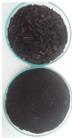
Fig. 3. Biochar from Sida hermaphrodita biomass obtained by pyrolysis at 400°C was used to fertilize sandy soil (on the right – after fragmentation).
