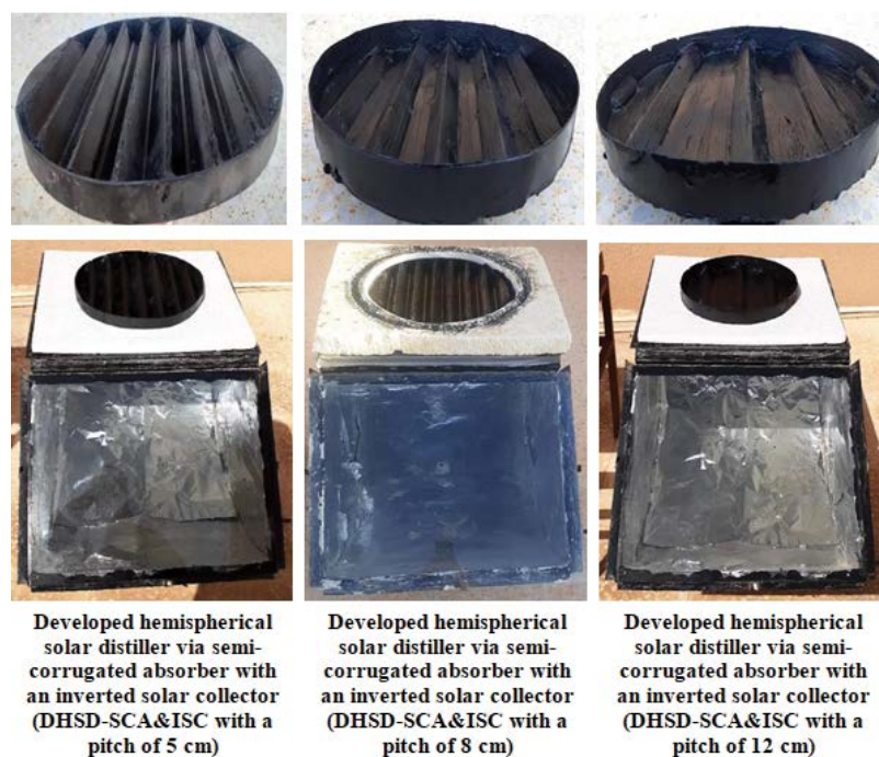
Fig. 2. A photograph of the basins of the developed hemispherical solar distiller via a semi-corrugated absorber combined with an inverted solar collector.
