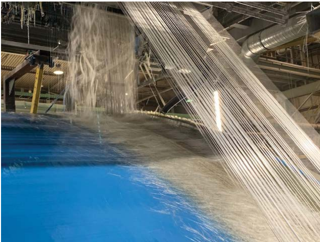
Fig. 7. Process of applying glass fibre to a non-circular profile [10].
