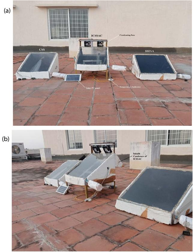
Fig. 2. (a) Experimental setup – CSS, SSIAA and ICSSAC. (b) Side view of experimental setup showing the inbuilt condenser in ICSSAC.
