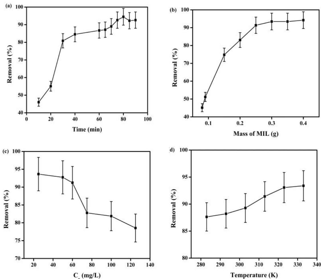
Fig. 3. (a) Effect of contact time, (b) dose of MIL powder, (c) initial eosin yellow concentration, and (d) temperature on eosin yellow release from wastewater.
