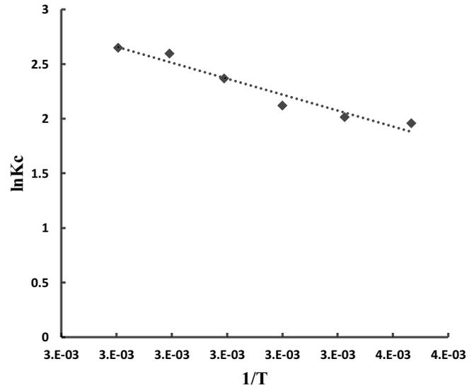
Fig. 7.  $1/T$  vs.  $\ln K_c$  plot regarding eosin yellow adsorption at MIL powder.
