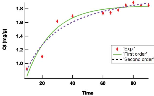
Fig. 6. Non-linear pseudo-first-order and pseudo-second-order kinetic plots regarding eosin yellow adsorption upon MIL powder from wastewater.
