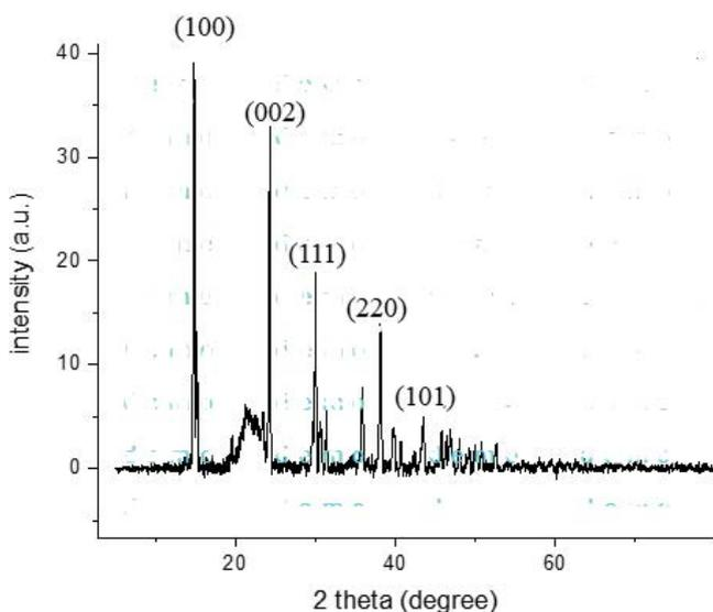
Fig. 2. X-ray diffraction pattern of MIL powder.
