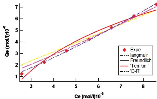
Fig. 4. Non-linear graph of Temkin, Langmuir, Dubinin–Radushkevich and Freundlich for adsorption of eosin yellow onto MIL powder from wastewater.
