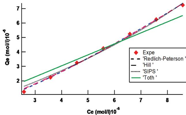
Fig. 5. Non-linear plots of Hill, Redlich–Peterson, Sips and Toth for the adsorption of eosin yellow onto mango leaves from wastewater.
