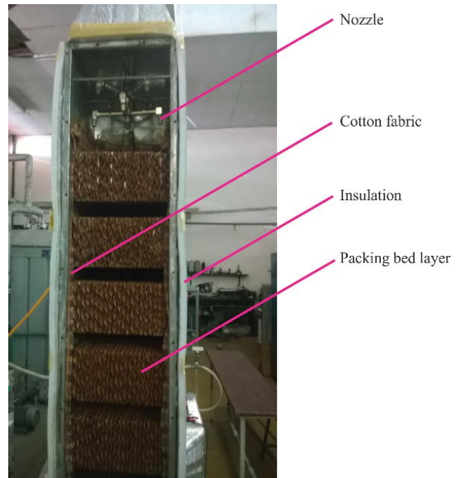
Fig. 4. Structure of humidifier.
