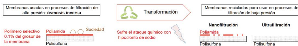
Fig. 5. Oxidation process of reverse osmosis membranes in nanofiltration or ultrafiltration membranes.
