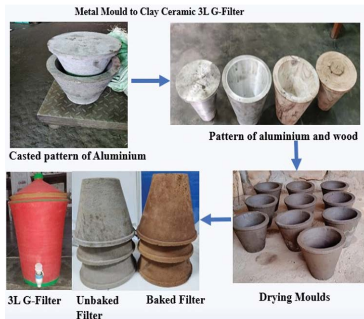
Fig. 1. Steps of manufacturing with a 3L G-filter.
