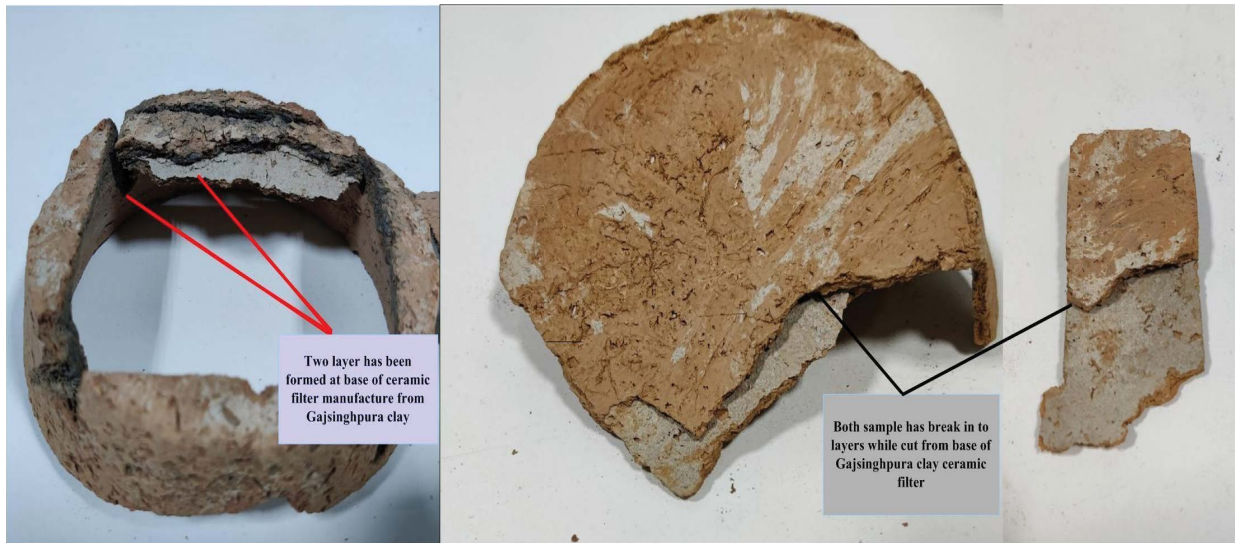
Fig. 13. Gajsinghpura soil based 3L G-filter base elaborating a layered fractured structure.
