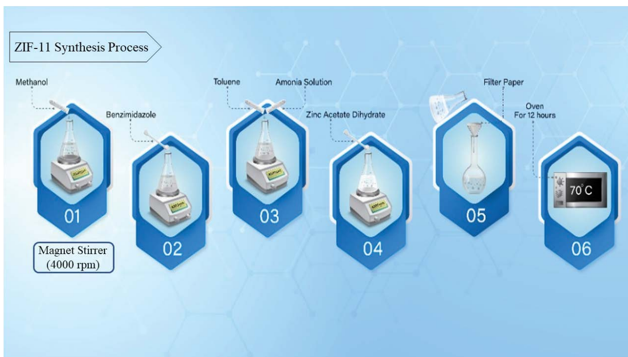
Fig. 1. ZIF-11 synthesis procedure.
