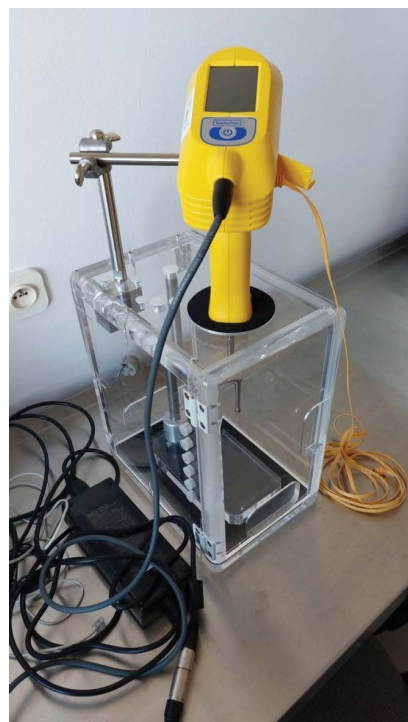
Fig. 1. Ultrasonic homogenizer by Hielscher Ultrasonics GmbH with the ultrasound frequency of 26 kHz (Author's photo).
