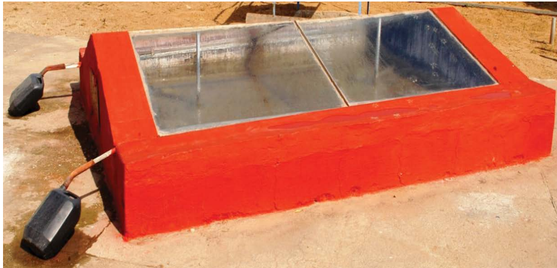
Fig. 2. Solar desalination devices made of brick-cement plastered material.
