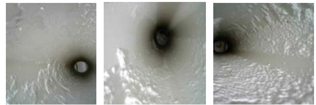
Fig. 9. Internal crystallization condition of pipeline under condition c (from left to right: pipe sections 1, 3, and 5).
