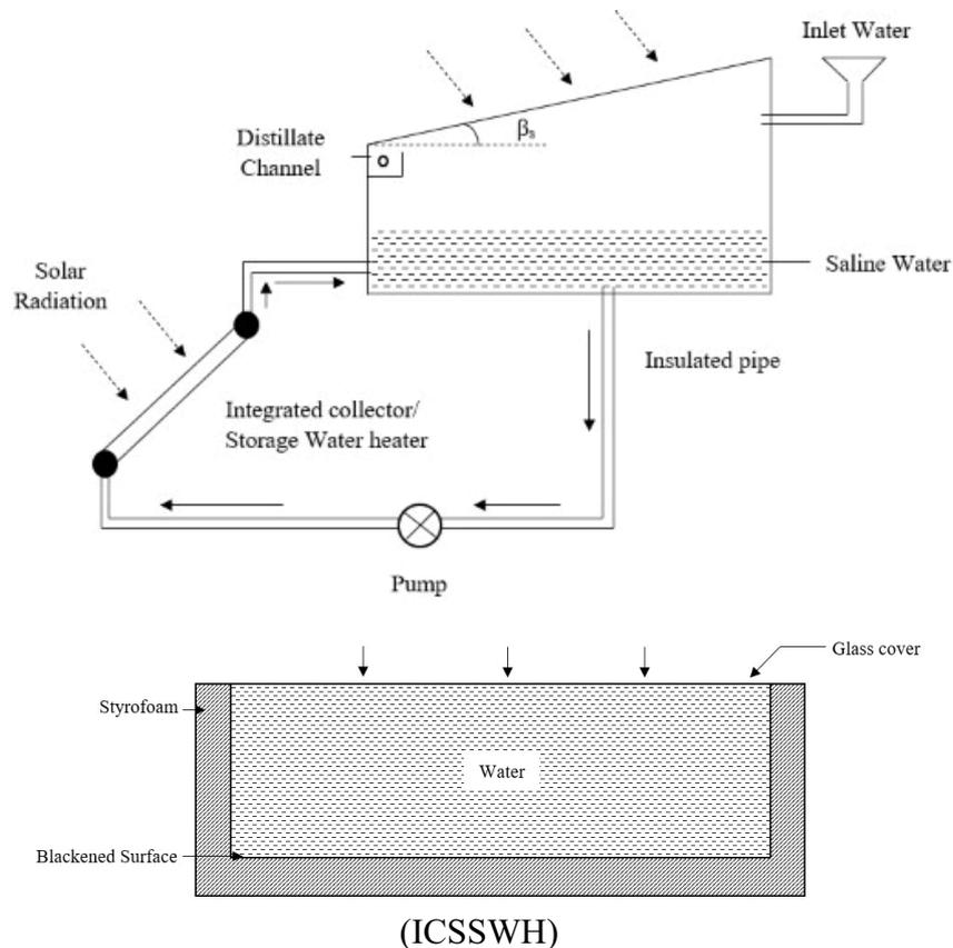
Fig. 2. Active single slope solar still coupled with ICSSWH.
