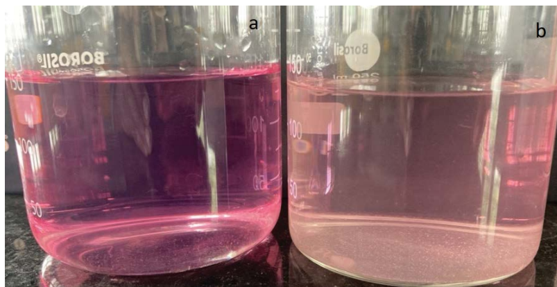
Fig. 9. Dye colour (a) before and (b) after photocatalytic treatment.
