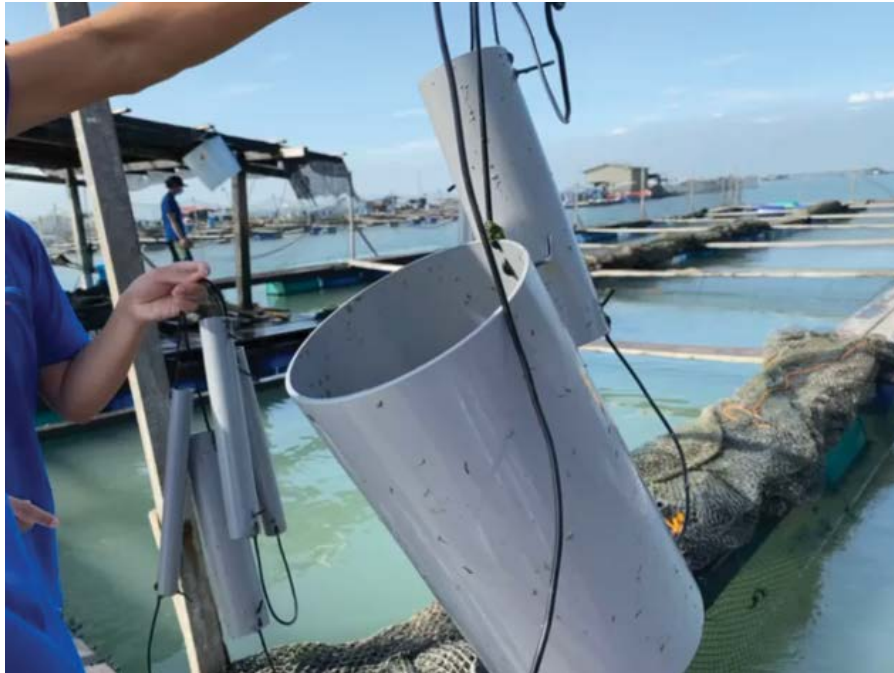
Fig. 8. Break and Protect 2 (BP2) marine leech trap device by Kua and Arbi [82] (Source: 3 Little Fish Malaysia).
