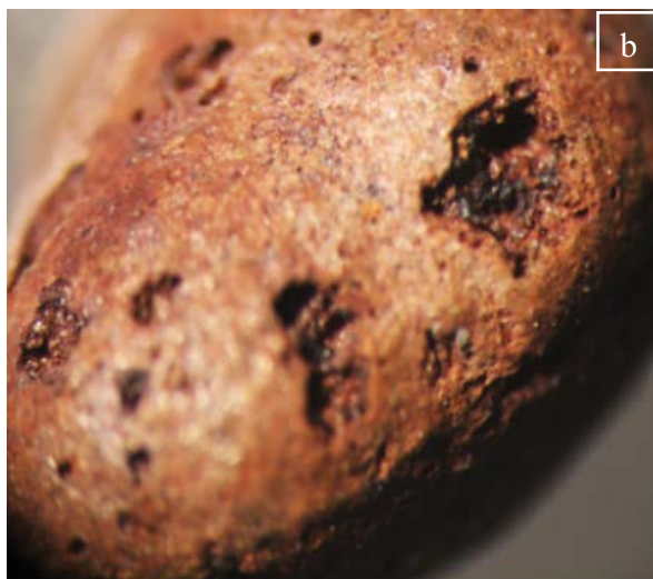
Fig. 2. (a) Scanning electron microscopy image of LECA particles and (b) binocular microscope image of \alpha\text{-Fe}_2\text{O}_3\text{@LECA} .
