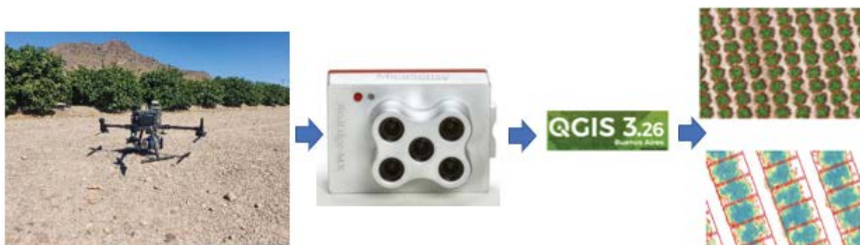
Fig. 8. Procedure for multispectral imaging for the generation of boron toxicity indicators.
