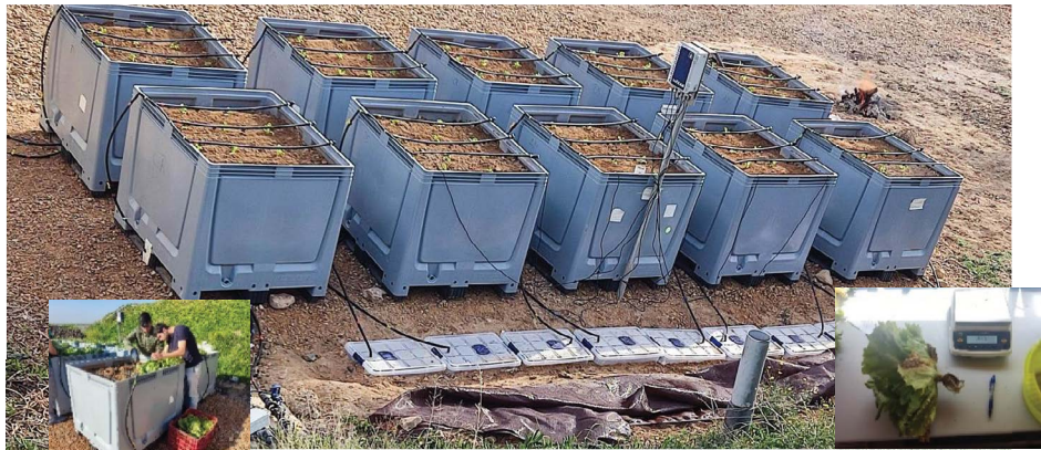
Fig. 6. Containers for analysis of boron phytotoxicity in annual crops located in the experimental plot of the SOS AGUA XXI project.
