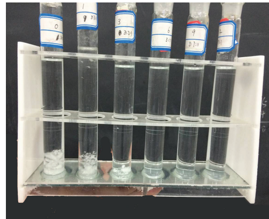
Fig. 8. Relationship between CaSO 4 scale inhibition efficiency in the presence of different inhibitor.
