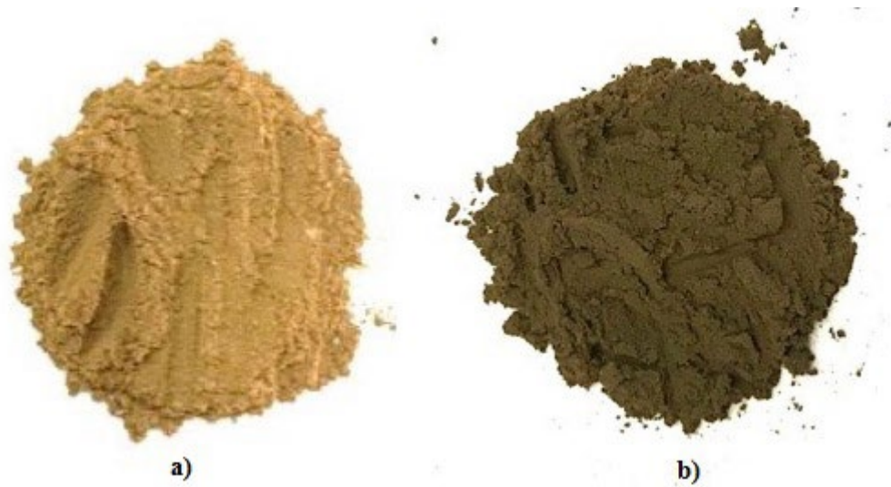
Fig. 3. Images of SC-FA-G2 (a) before and (b) after the RB19 dye adsorption process.
