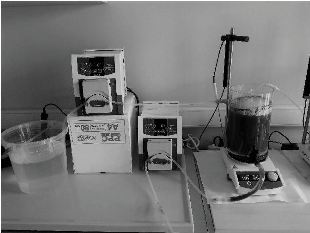
Fig. 2. Lab-scale completely mixed continuous flow reactor.
