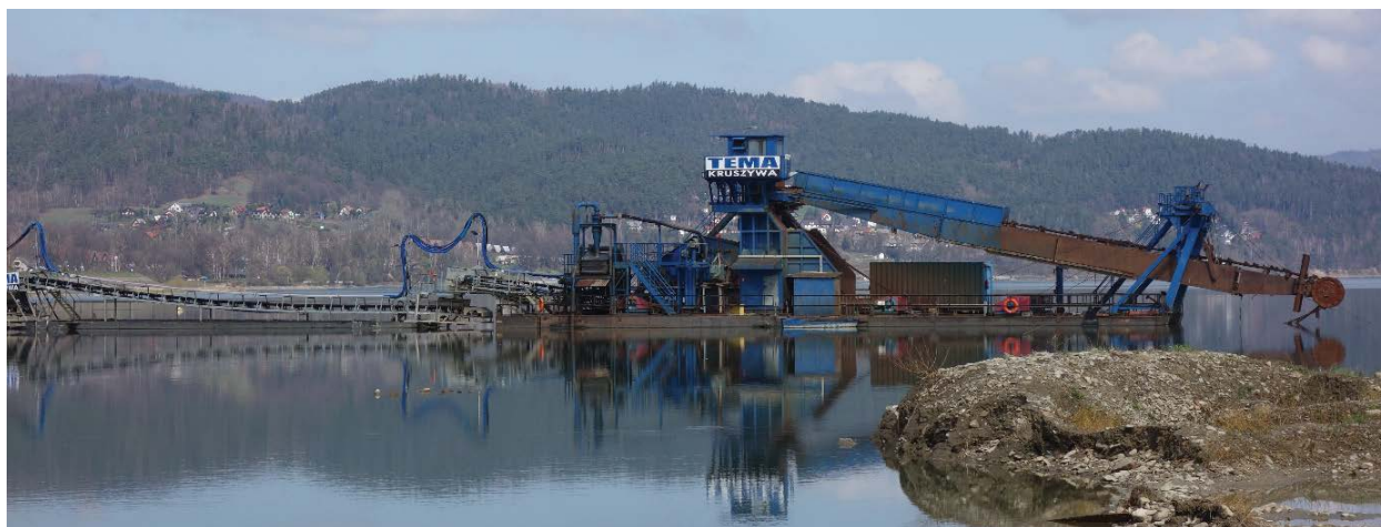
Fig. 2. Multi-bucket dredger in the Tresna Reservoir (photo by A. Jaguś).
