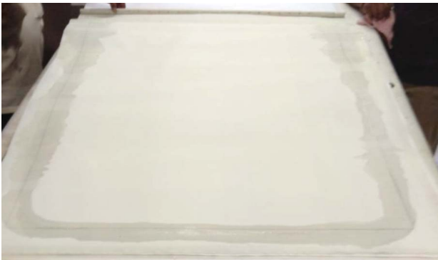
Fig. 5. Adhesive lines as observed when the module was reopened for observation after applying winding pressure. Application of the winding pressure ensures that the adhesive has spread in the free space.
