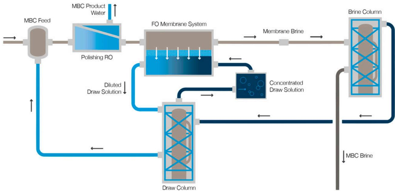
Fig. 6. Process flow schematic for the Changxing Power Plant MBC, including the preconcentration/polish RO membrane system, FO membrane system, and thermal draw recovery system. The primary difference between this process and the standard MBC is the preconcentration RO step used to treat the low TDS feedwater and improve overall process economics.
