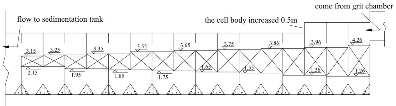
Fig. 7. The modification diagrammatic sketch of the reaction tank.
