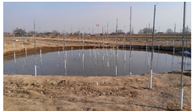
Fig. 4. Overview of the test pit for the filed soaking test.
