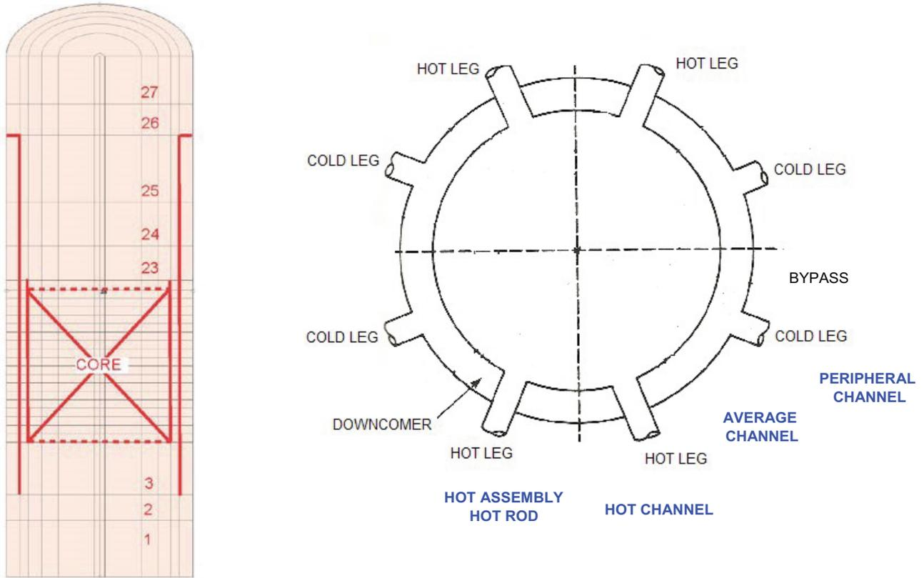
Fig. 2. 3-D nodalization for RPV.
