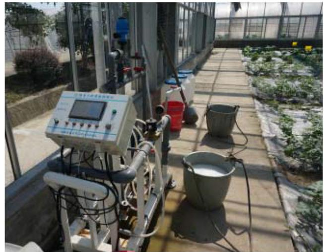
Fig. 11. Water–fertilizer irrigation control equipment and demonstration.
