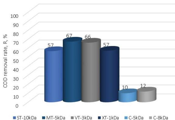
Fig. 10. COD removal by UF process with PES and ceramic membranes.
