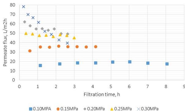
Fig. 6. Permeate flux for XT-1 kDa membrane as a function of transmembrane pressure in the range of 0.1–0.3 MPa.
