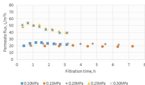
Fig. 3. Permeate flux for ST-10 kDa membrane as a function of transmembrane pressure in the range of 0.1–0.3 MPa.
