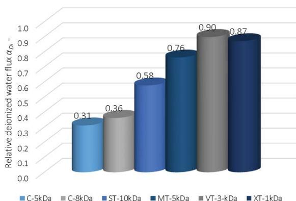
Fig. 9. Relative deionized water flux through polymeric and ceramic membranes applied in treatment of biological effluents.
