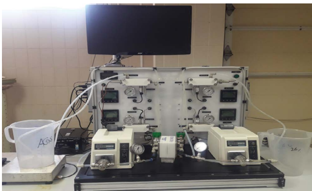
Fig. 1. Laboratory-scale forward osmosis instrument.
